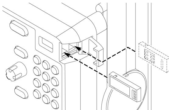
Refer to the drawing. With the instrument off, insert the MDO3BND application module into one of the two available application module slots. The MDO3BND application module will enable each application module included in the bundle.
